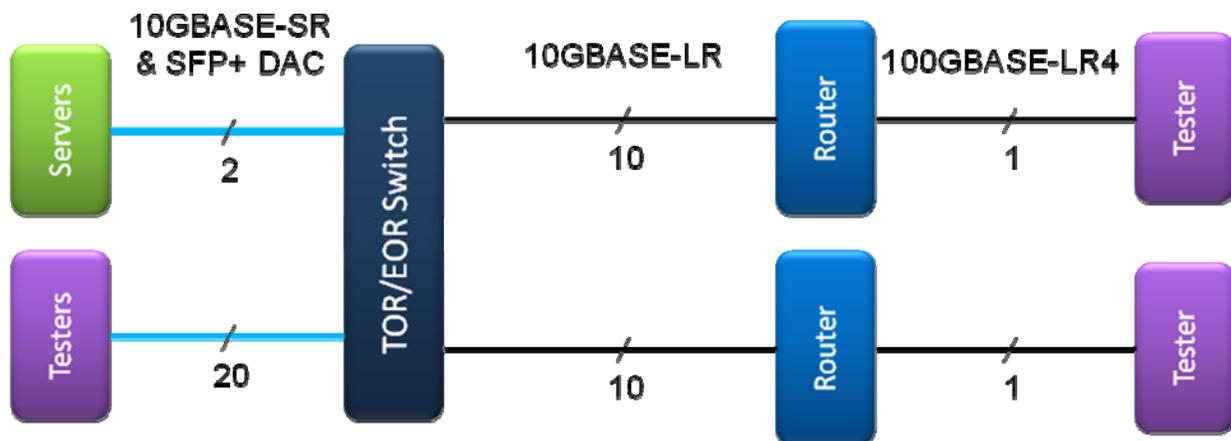
Starting on the left, the Ixia XM12 tester is equipped with 16 ports of 10GbE using the SFP+ form factor, and the Spirent TestCenter tester is equipped with 8 ports of 10GbE also using the SFP+ form factor. Mellanox Vantage 6048 top-of-rack/end-of-row (TOR/EOR) switch is equipped with 48 ports of SFP+, and each port on the switch is capable of operating in either 1GbE or 10GbE mode. For this demonstration, the switch operated all its ports in 10GbE mode.
