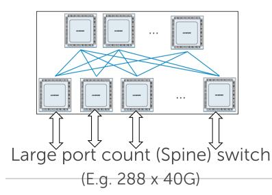
Data center scale-out ~ O(F^2); F = switch radix
