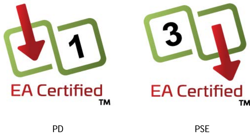
Figure 2: The EA CERTIFIED logo on the left indicates a Class 1 PD, and the logo on the right indicates a Class 3 PSE. The classification number makes it easy to see when a PSE will fully power a PD (if PSE class is greater than or equal to the PD class).
