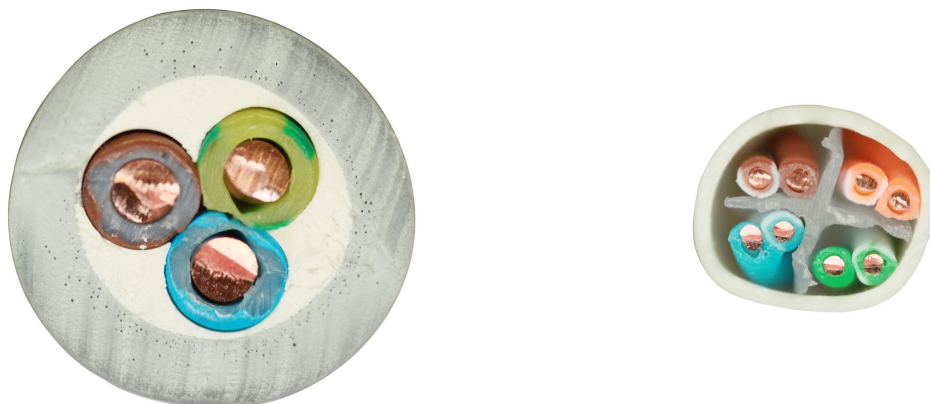
Figure 1: Cross section of 2.5 mm 2 solid copper mains wire, next to solid copper 23 AWG CAT6 cable at the same scale.
