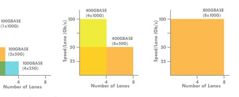
Total throughput (data rate) may be achieved in three general ways, and combinations of them: Aggregating multiple lanes 2 Increasing the per lane bit rate
